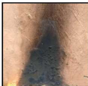
Fig. 8: Second pattern formed on the vertical wall after kerosene was spilled and then burned.
