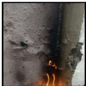
Fig. 7: First pattern formed on the vertical wall after kerosene was spilled and then burned.
