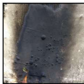
Fig. 9: Third pattern formed on the vertical wall after kerosene was spilled and then burned.
