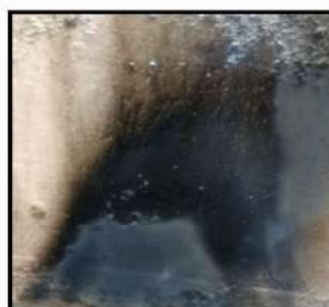
Fig. 5: Second pattern formed on the vertical wall after diesel was spilled and then burned.
