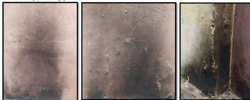
Fig. 1: First pattern formed on the vertical wall after petrol was spilled and then burned.
