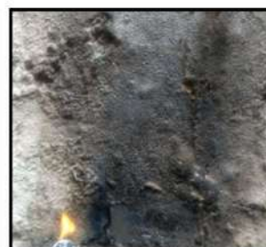
Fig. 6: Third pattern formed on the vertical wall after diesel was spilled and then burned.
